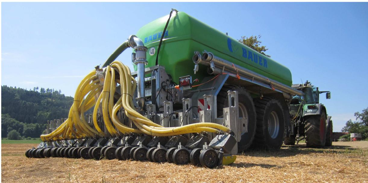
Image caption: Bauer CerresX slot slurry injector
