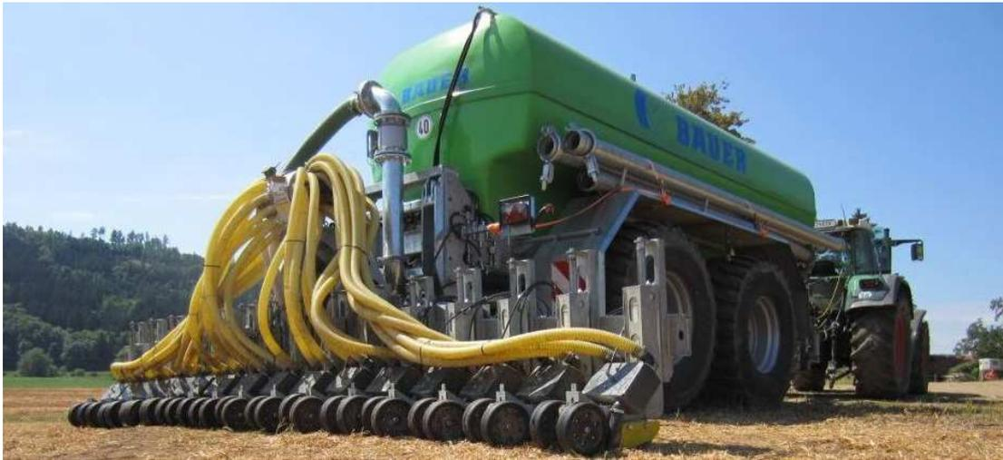
Image caption: Bauer slurry trench machine CERRES-X
